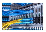
Fiber Optic Cables: Ideal for long-distance communication and high-speed data transfer. Immune to electromagnetic interference, making them suitable for industrial environments.
